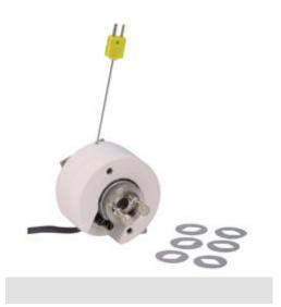
Heat is applied through a heater band and regulated by a temperature controller, which must be purchased separately. A Chromel-Alumel K-type thermocouple is provided for continuous monitoring of the temperature (up to 400°C) on the inside of the sample chamber.
